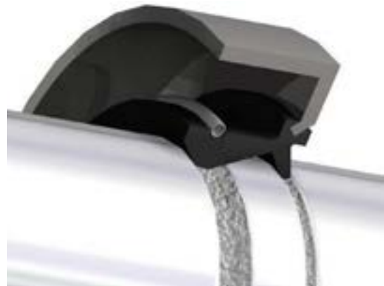
Figure 5: Fluid media passed through rotating unions with soft seals must be kept free of contamination to prevent suspended particles from embedding in the seal and damaging the rotor.
