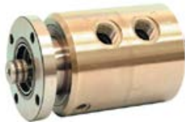
Figure 6: Deublin's hydrostatic sealing technology features precisely engineered gaps between the rotating union's rotor and bushing, through which a thin film of bypass fluid flows to lubricate the assembly.
