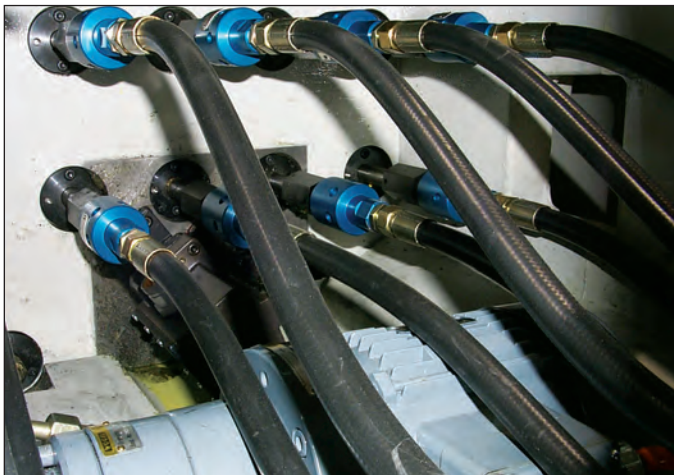
Deublin 1116 Bearing-Supported Unions on Automotive Transfer Line.
