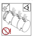
Check the union for leakage. A small amount of leakage may occur in the starting period.
