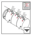
Passages may be media-specific or function-specific, depending on the union model. Make sure that passages are connected correctly by checking the DEUBLIN IC drawing.
