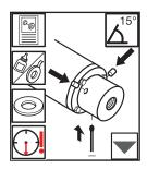
Connect the drain hose (at least 8 mm cross section) at the union. If the union is used horizontally, the drain port must be in 6 o'clock position. Drain hose should slope down regardless of union orientation (horizontal, vertical, or other). Drain hose must be flexible. Close the rest of the leakage bores with the plugs delivered with the union.
