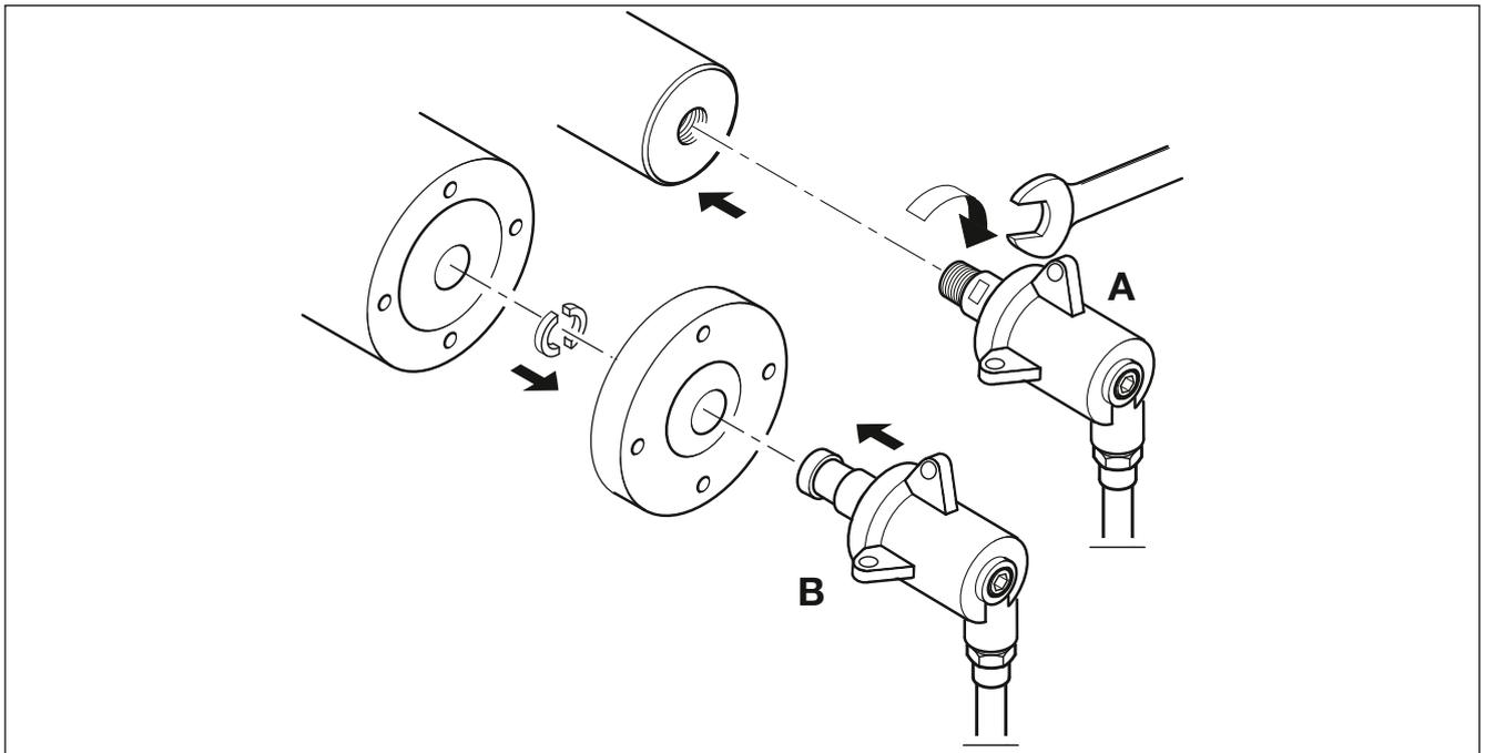
Fig. 4: Options for the installation on the machine shaft
