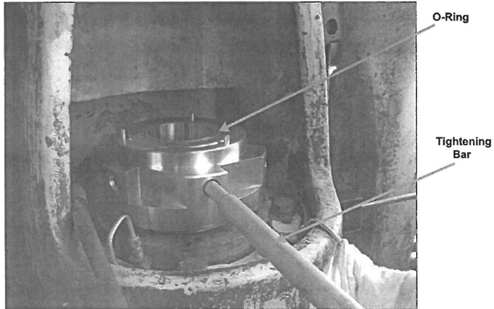
Figure 3-5. Installing the Lower Nut
