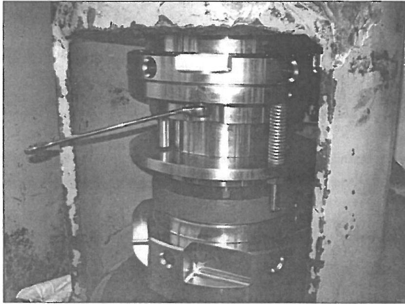
Figure 3-10. Tightening the Cap Screws
