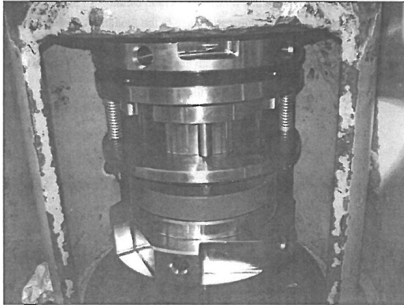
Figure 3-9. Lining up Holes for the Cap Screws
