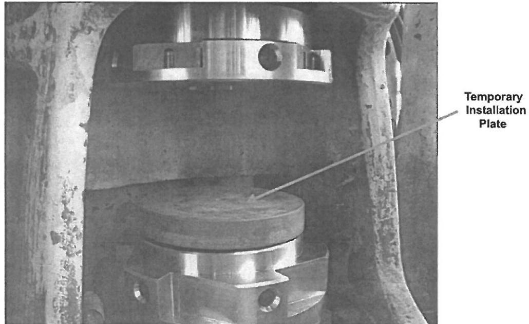
Figure 3-7. Positioning Temporary Installation Plate
