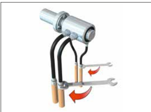
Fig. 5: Connect hoses with straight connections
