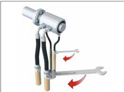
Fig. 4: Connect hoses with 90° elbows
