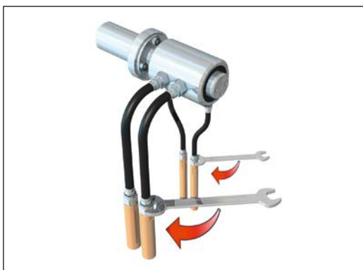
Fig. 7: Connect hoses with straight connections
