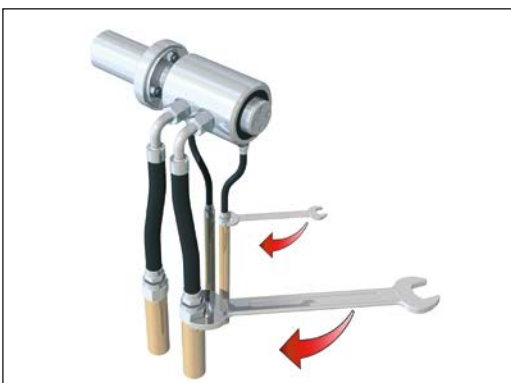
Fig. 6: Connect hoses with 90° elbows
