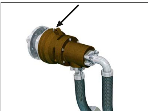
Fig. 8: Attach grease gun for relubrication
