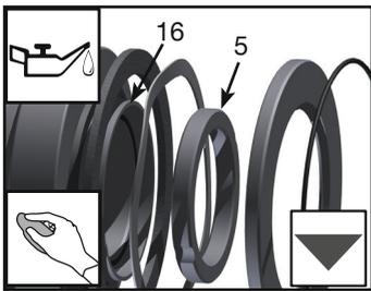
Make sure lubricated (TS10) new O-Ring (16) is seated on rotor before installing the new seal face (5). Wipe-clean (TS6) both sealing surfaces on the seal (5) and seal kit sub-assembly (9) with alcohol (TS5). Put a few drops of clean lubrication oil (TS7) on the seal face (5) and (9) surface.
